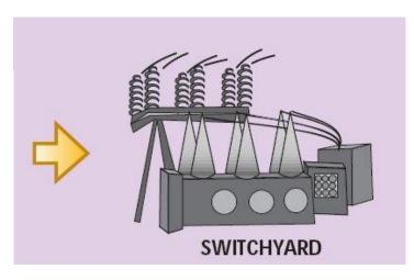
The electricity moves from the generator to a switchyard at the power plant. There it is transformed to a higher voltage and sent on its way via a transmission line. Transmission lines generally are rated at 69,000 to 500,000 volts (compared to 120 - 240 volts in your home)
